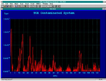
**Analog mode** provides a line graph representation of the acquired mass spectrum (partial pressure vs. mass number). Span, resolution and noise floor can each be set. Scans can be single-shot, timed or taken continuously.
