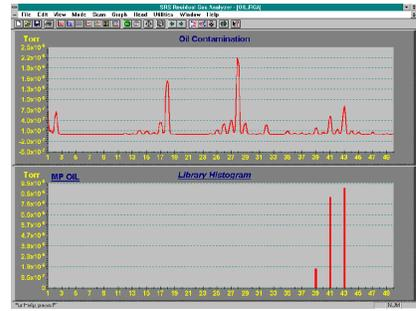
**Library mode** contains a comprehensive list of gases that can be used to compare against the current spectrum. A search mode allows you to select up to 12 masses and identify and display (numerically and graphically) the intensity of all gases that contain these masses.
