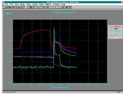
**Pressure vs. time** presents a strip chart of partial pressures for selected masses and provides a complete time history of your data. Complete scrolling and zoom control is available even while data is being acquired. This mode is most often used for monitoring process trends.
