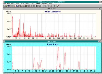
**Multi-head operation** is available when when more than one RGA is needed for analysis. Up to eight heads can be monitored simultaneously from the software.
