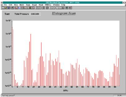
**Histogram mode** displays a bar graph of partial pressure vs. mass, allowing the spectrum to easily be interpreted. This mode is often used for quick and easy vacuum analysis. The screen can be split for viewing two modes of operation simultaneously.
