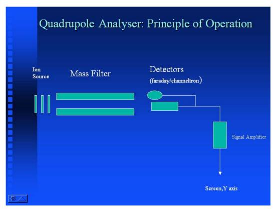
Ions emerging from the source region will encounter the quadrupole rod set or "Mass Filter" system.
