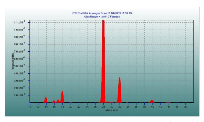
The spectra shown above represents a typical result from a Residual Gas Analyser, a number of Gaussian peaks centred on a mass position, with good separation (resolution) and differing intensities. The spectrum represents components within a vacuum system which are often referred to as "Partial Pressures".
