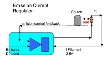
The emission current regulator operates by sensing the electron emission current between filament and ion source compared to a fixed demand input. The large *heating current* in the filament is regulated in order to maintain the desired *emission current*.
